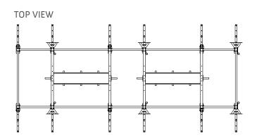
Note: X-Racks are required to be bolted to a concrete sub-floor
